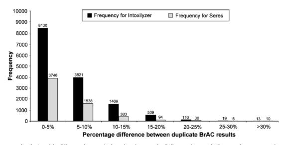
FIG. 2—Frequency distribution of the differences between duplicate breath test results. Differences between duplicate results are expressed as a percentage of the lower result.
